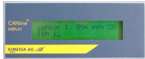
Display view in case of alarm.
